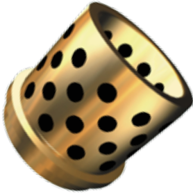
BRONZE with SELF-LUBRICATING GRAPHITE PLUGS
