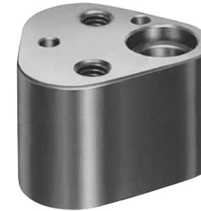
Pilots are critical tools used in a die set—ones that can ultimately determine the quality of a stamping or fabricating operation. Because they are the primary locating devices, pilots need to be mounted properly to avoid unwanted lateral deflection. As bending or forming of the metal takes place, this lateral deflection can create excessive force on the pilot. Often, the strength of the pilot—as well as the function of the other die set components—is compromised.
