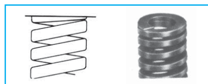
Ends of each spring are closed and ground square to assure that the spring will stand on either end and provide a maximum bearing surface.
